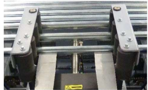
Motorized side guide rollers with idle conveyor rollers for 0.25" base
